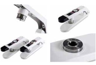
**CALIBRATION:** Each new ST300 supplied is calibrated by MSA to the full requirements of ISO 17235:2015. MSA also offers a comprehensive re-calibration service.
